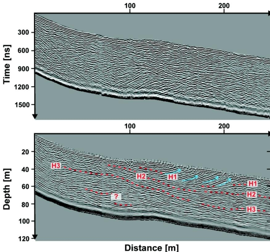
**FIGURE 16:** Unmigrated (upper row) and migrated (bottom row) radargram sections of GPR profile 1. Migration velocity was 0.14 m/ns. Broken lines are interpreted horizons. H2 probably marks the base of the massive ice core which is up to about 30 m thick. H3 has a maximum depth of 45 m and is caused by the surface of the bedrock. Between 120 and 210 m concave shaped reflection bands are well developed. Between H2 and H3 unfrozen debris is present.
