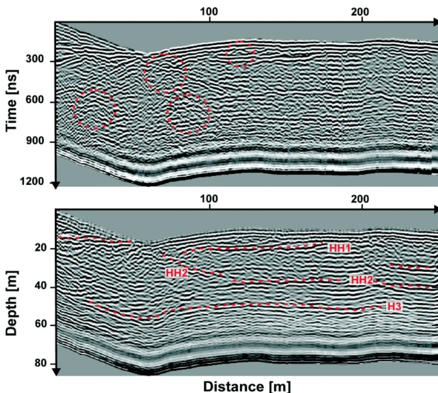
**FIGURE 18:** Unmigrated (upper row) and migrated (bottom row) radargram sections of GPR profile 3. Migration velocity was 0.14 m/ns. Broken lines are interpreted horizons. Circles indicate pronounced diffraction hyperbola. HH2 probably reflects the base of the frozen core of the rock glacier which is composed of a mixture of debris and ice. H3 is interpreted to represent the surface of the bedrock.
